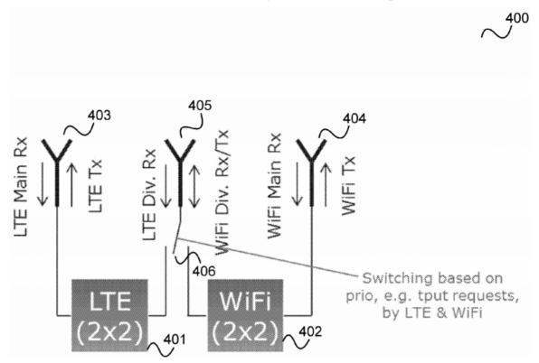
Clevorn's Figure 4 illustrates first antenna 403, which is permanently assigned to LTE transceiver 401, second antenna 405—which through switch 406 can be switched between LTE transceiver 401 and WiFi transceiver 402—and third antenna 404, which is permanently assigned to WiFi transceiver 402. Clevorn ¶ 87.
