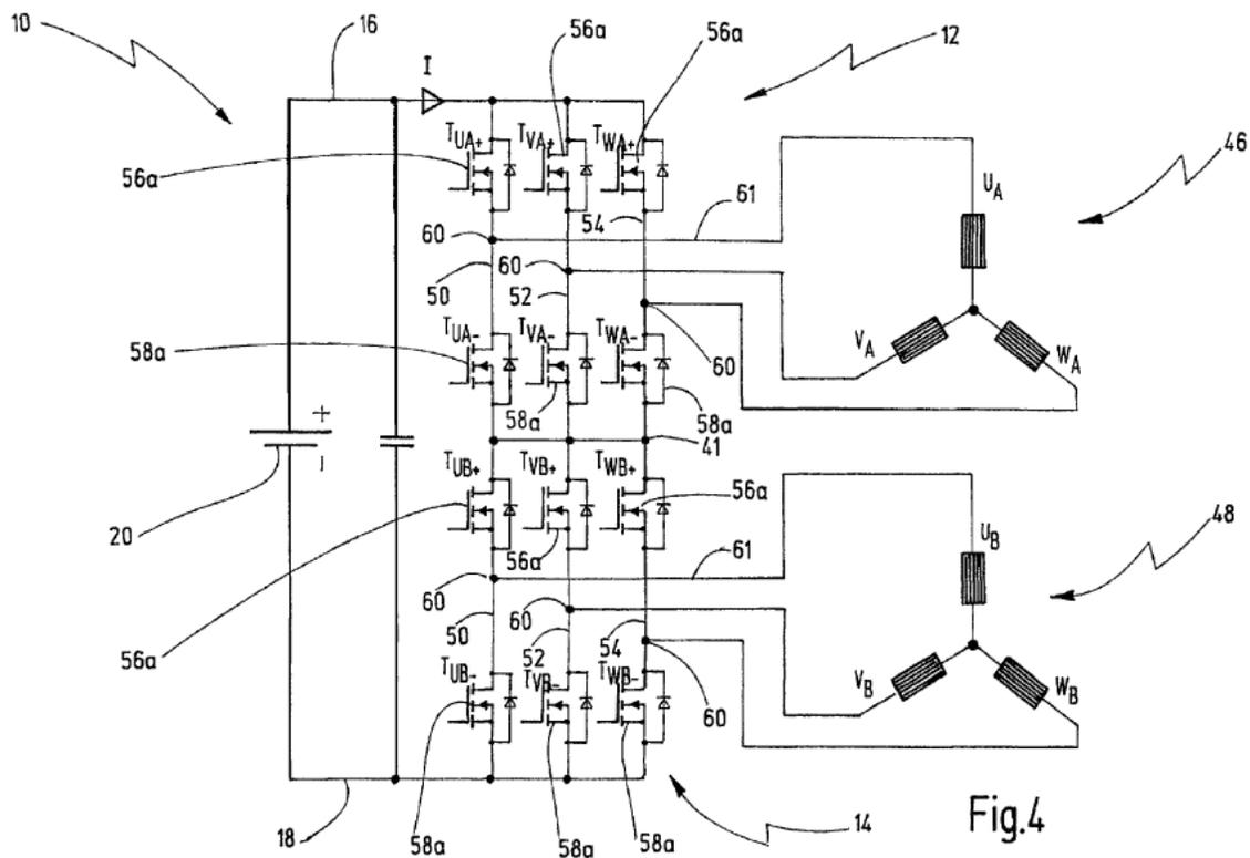
Figure 4 is a schematic circuit diagram of a control unit having controllable semiconductor switches
