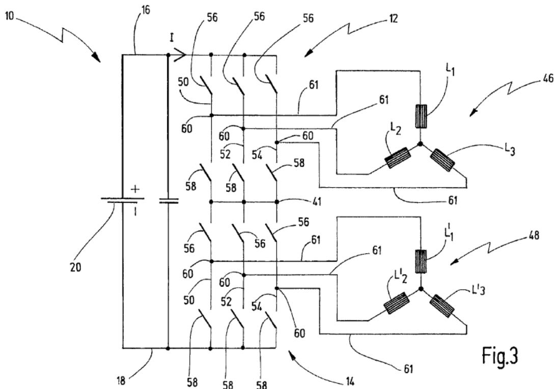
Figure 3 is a schematic circuit diagram of a control unit for controlling two coil arrangements of an electric drive
