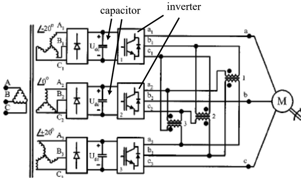
Fig. 5. Cascaded inverter with three-phase cells.
