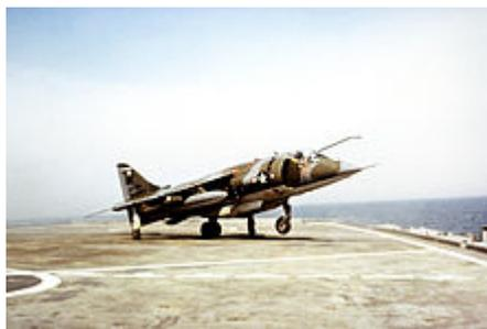
AV-8C Harrier taking off from an amphibious transport dock ship
