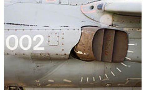
Thrust vectoring nozzle on a Sea Harrier
