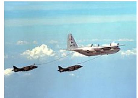
A pair of USMC AV-8A Harriers refuelling from a Lockheed Martin KC-130 tanker
