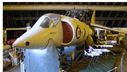
Former Harrier GR.1 that crashed in 1971 and used as a static engine test bed by Rolls-Royce, seen on display at the Bristol Aero Collection, Kemble, England
