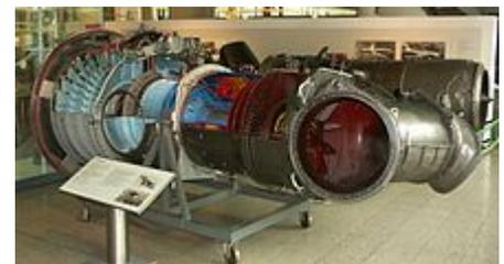
Rolls-Royce Pegasus engine on display, sections have been cut out to provide an internal view
