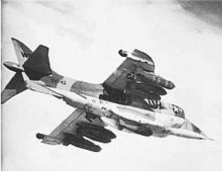
An RAF Harrier GR.1, on loan to the USMC, displaying its underside with a full load of bombs
