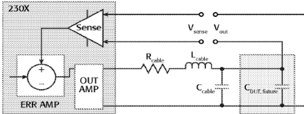
Keithley Figure 2 is a “Simplified Series 2300 measurement schematic with reactive load and remote-sense feedback.” *Id.* at col. 2.
