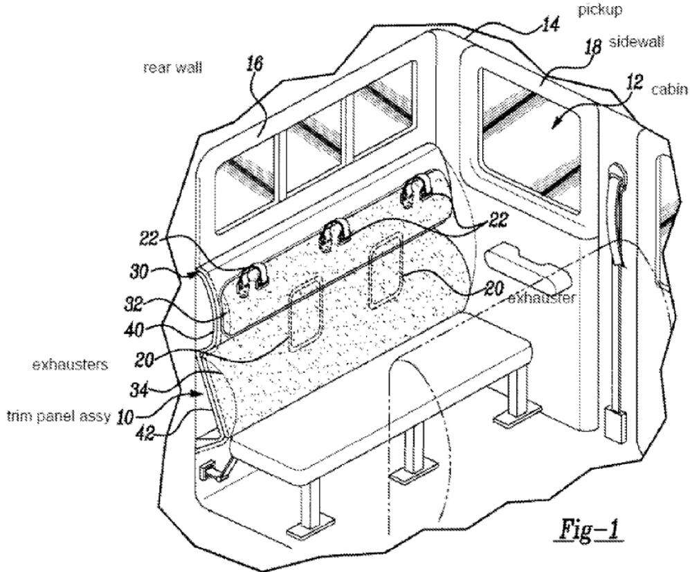
Annotated Figure 1 of Gac '677 is a perspective view of the interior of the back of a passenger cabin of a truck depicting exhausters 20 and much larger trim panel assembly 10 (on which insulating member 35 is located). See Ans. 5; Gac '677 5: 44-45, 3:26-29.
