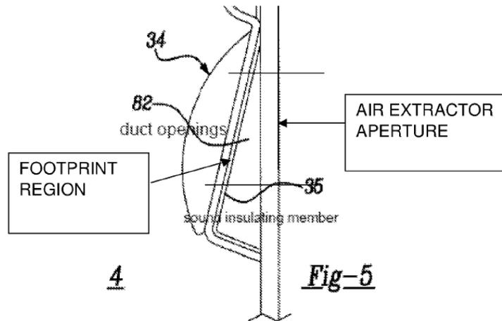
Annotated Figure 5 of Gac '677 is a partial cross-section of a trim panel assembly 10 depicting insulating member 35, and, via two unlabeled
