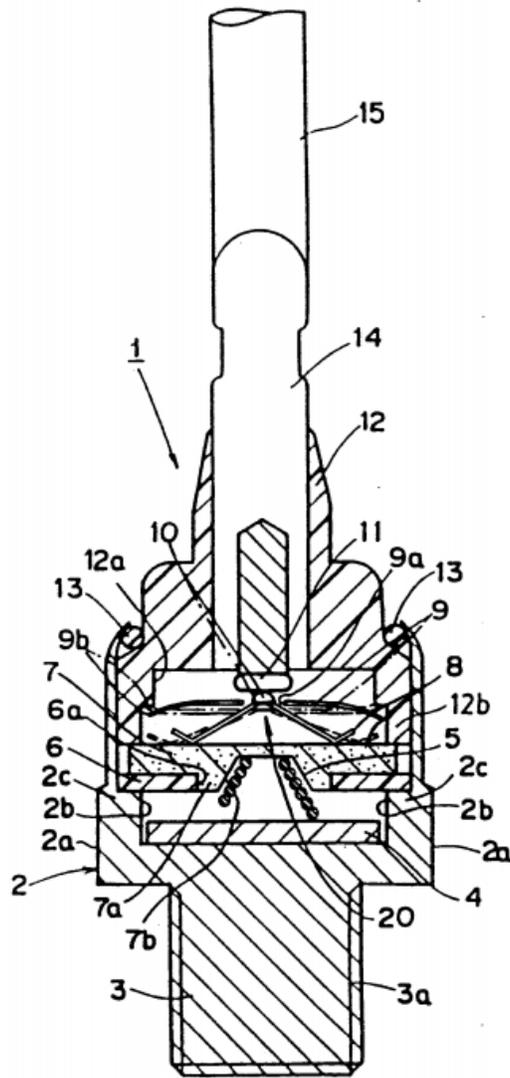
Figure 1 is a cross-sectional view of a heating device. Yamashita, 3:66–67. It shows disc-shaped heating element 4, conductive spring 5, insulating plate 6, conductive plate 7, and tripod spring 8, as well as movable contact 10 and stationary contact 11. *Id.* at 3:21–32, 3:44–56.
