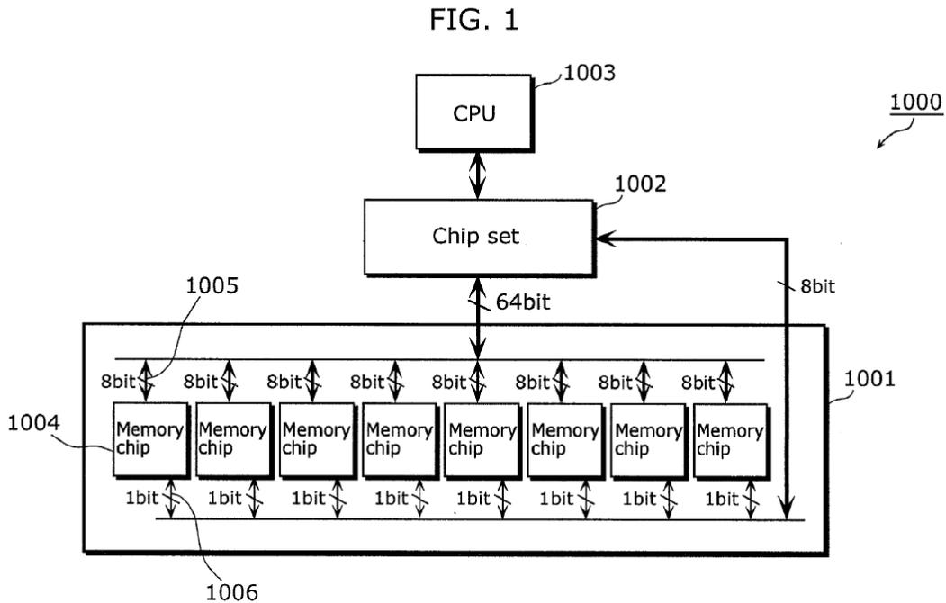
*Figure 1 is a diagram showing a configuration of a conventional computer system.*
