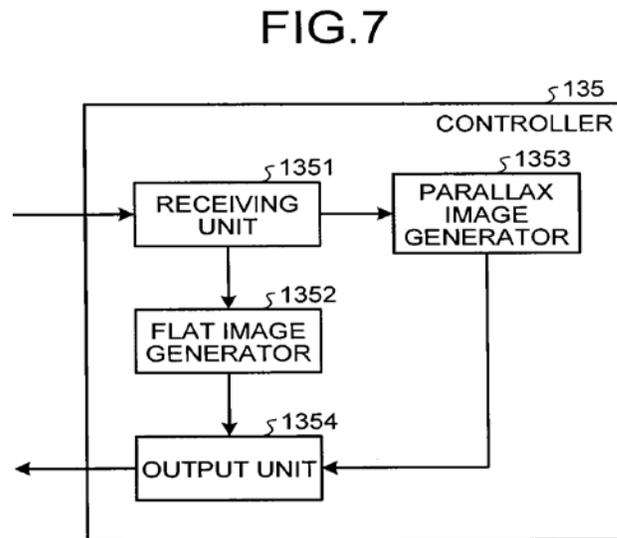
Figure 7 illustrates a controller within workstation (Fig. 4, 130) of image processing system (Fig. 1). *Id.* at 21–22.
