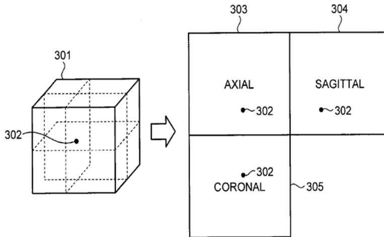
Figure 8 illustrates generated flat image (303, 304, 305) setting arbitrary coordinate point (302) on a stereoscopic 3D image of subject (301). *Id.* at 29: 8–10.
