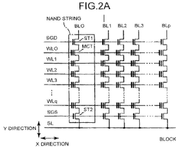
Figure 2A depicts a circuit diagram showing an example of a configuration of a physical block included in the NAND memory. *Id.* ¶¶ 5, 43.
