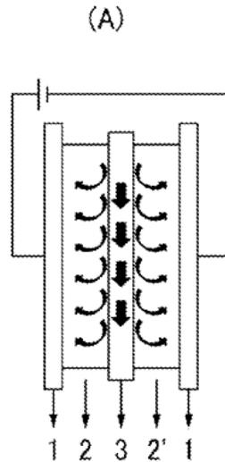
Figure 1(A) is a schematic view of an exemplary capacitive deionization apparatus
