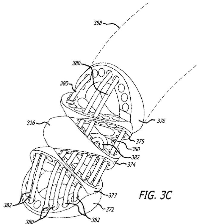
Figure 3C of Rogers which is a perspective view of a portion of the flexible shaft of a robotic surgical tool.
