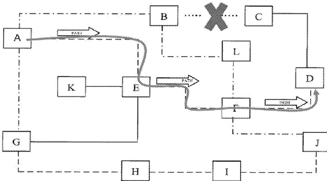
Fant’s Figure 5 shows an optical network where a primary path A-B-C-D fails, connection A→D is switched to a secondary path A-E-F-D.
