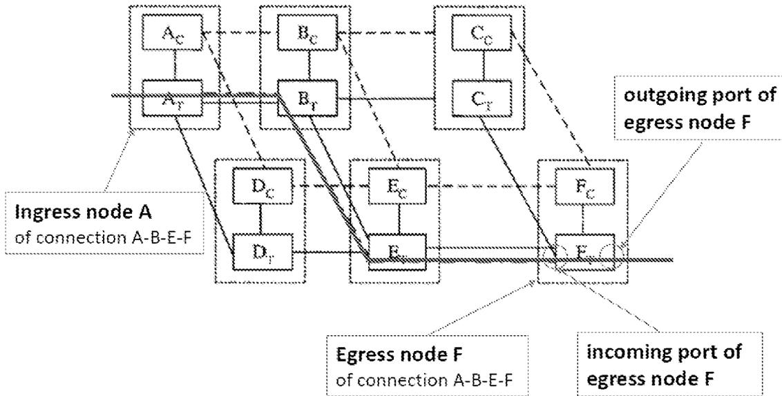
Wu's Figure 1 shows an optical network including, for example, six (6) nodes A–F connected via optical links to operate in [1] a data (transmission) plane AT–FT and [2] a control plane AC–FC (that can be physically combined but are logically separated) to establish connections (optical links) between nodes.
